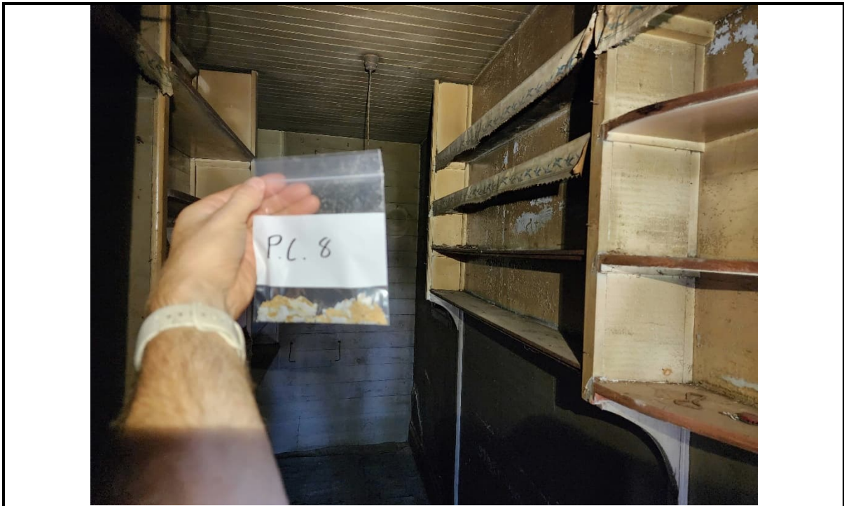
Photo 14: PC 8: Confirmed lead-containing cream paint in the pantry.
