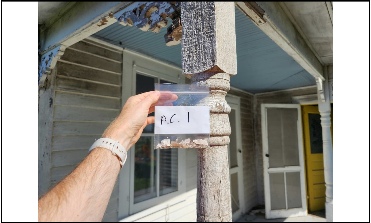
Photo 7: PC 1: Confirmed lead-containing white paint on an exterior wood post.
