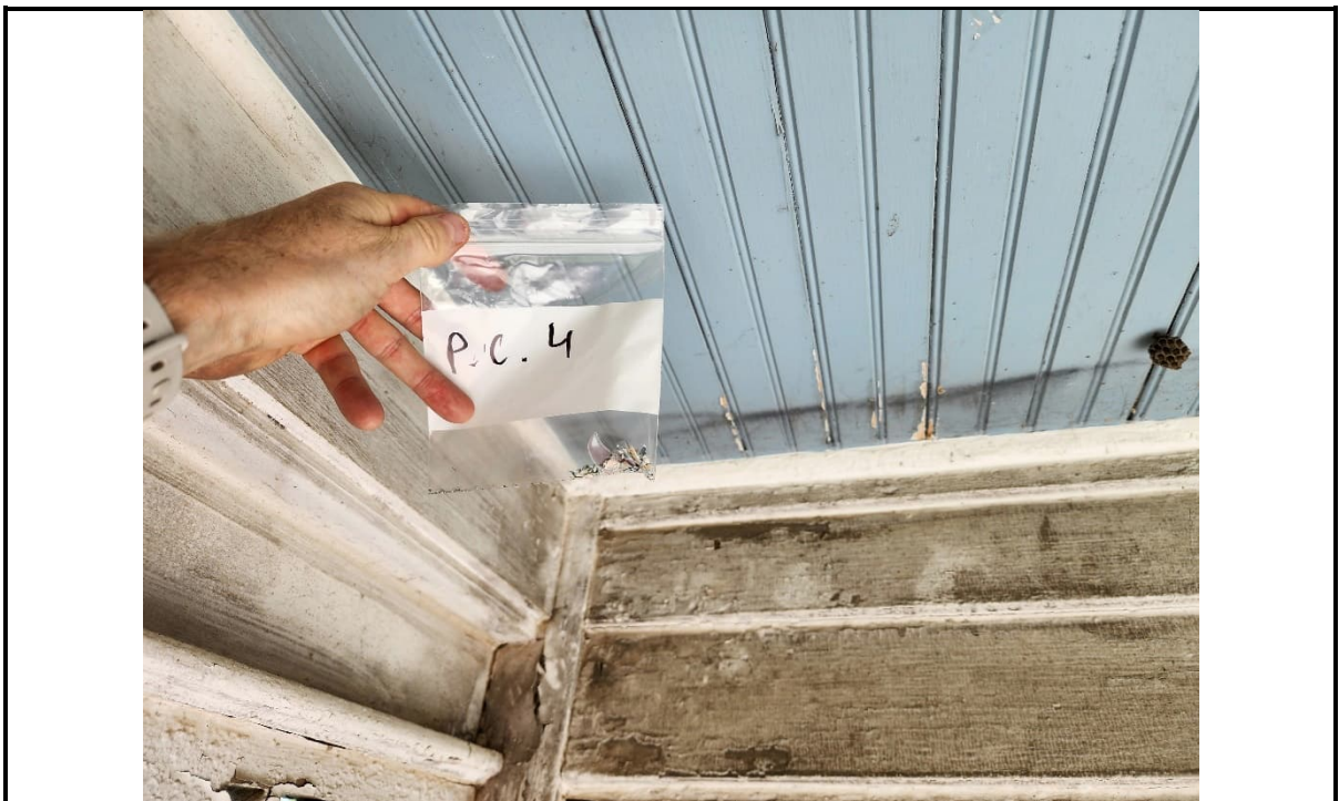
Photo 10: PC 4: Confirmed lead-containing blue paint on the front porch soffit.
