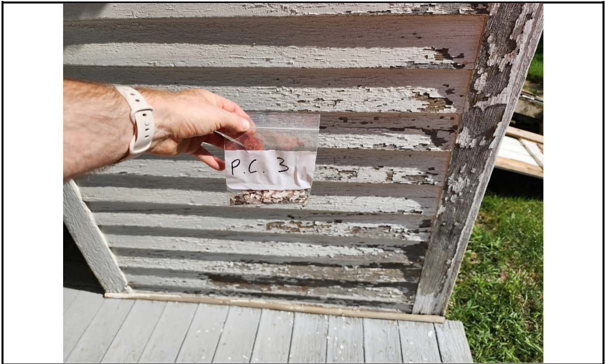
Photo 9: PC 3: Confirmed lead-containing white paint on the house siding.
