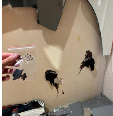
Photo #2 A-85 BR 165 Men's Room 1 st Floor, Black Mastic Puck behind mirror ( 5% Chrysotile ).
