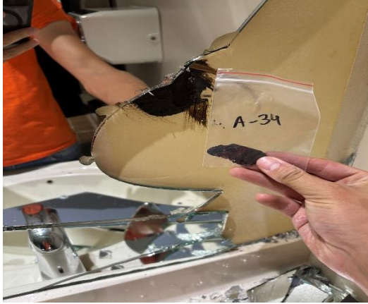
Photo #1 A-34 BR 363 Women Bathroom 3 rd Floor, Black Mastic Puck behind mirror ( 20% Chrysotile ).
