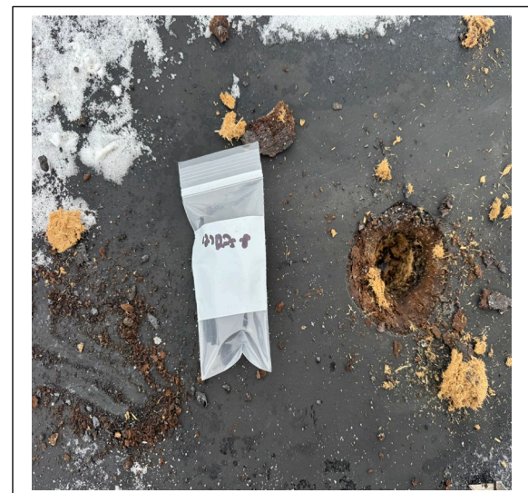
Sample 121225-8: Rubber/adhesive on West edge of main roof negative for asbestos.
