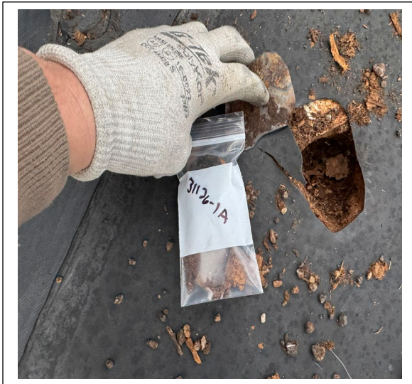
Sample 31126-1A: Field on canopy roof negative for asbestos.
