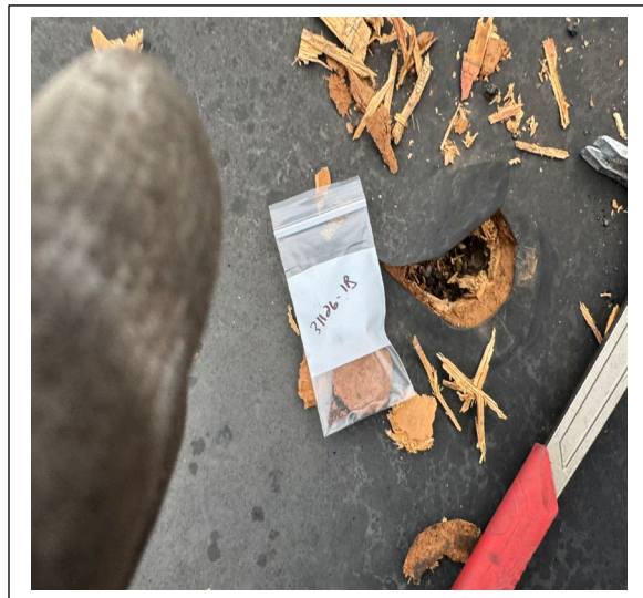
Sample 31126-1B: Field on canopy roof negative for asbestos.
