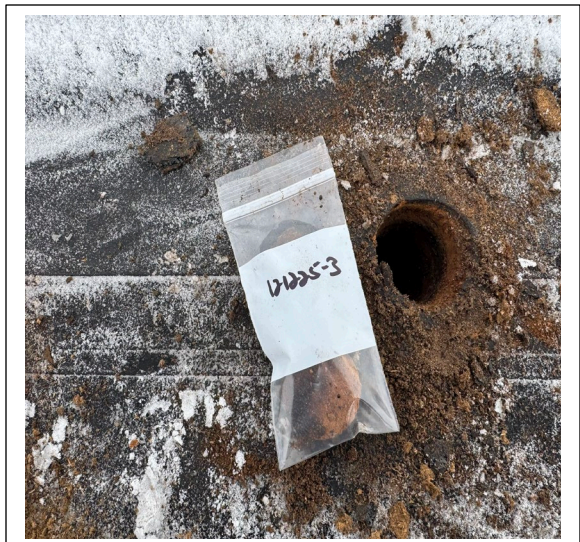
Sample 121225-3: Flashing on East edge, main roof of warehouse negative for asbestos.
