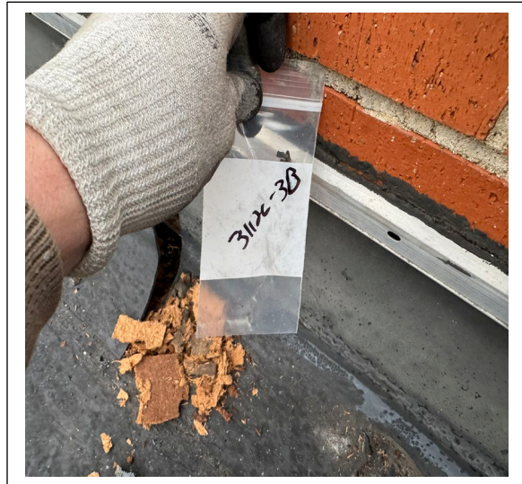
Sample 31126-3B: Caulking on flashing termination bar negative for asbestos.
