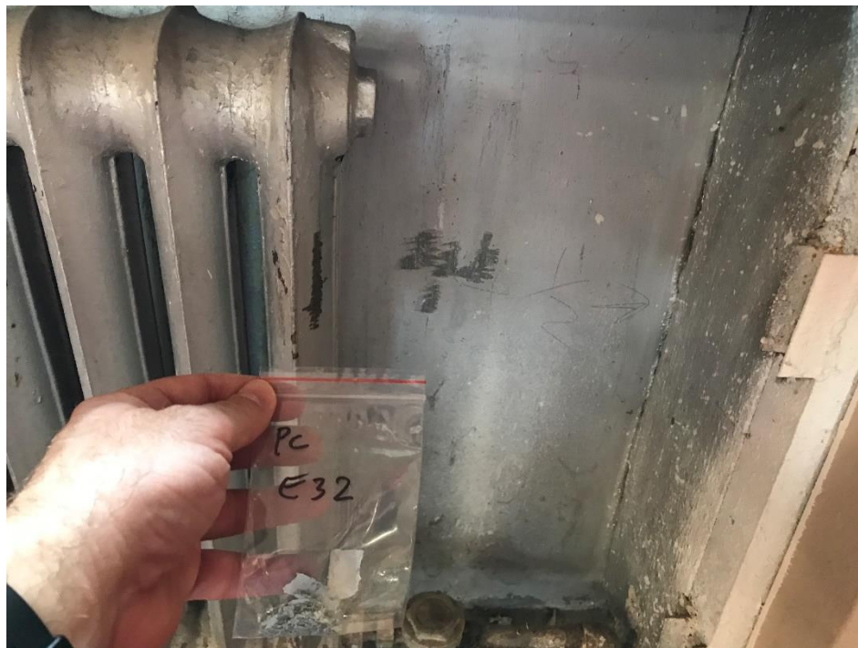
View of the Silver Lead Containing Paint. (PC E 32, 0.22% Pb)
