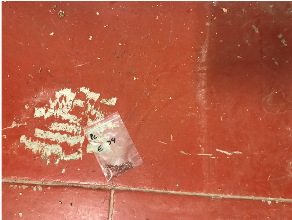
View of the Red Lead Based Paint. (PC E 34, 0.79% Pb)
