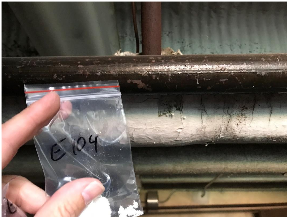
View of the Asbestos Containing TSI Run. (E 103, 10% Amosite & 10% Chrysotile)
