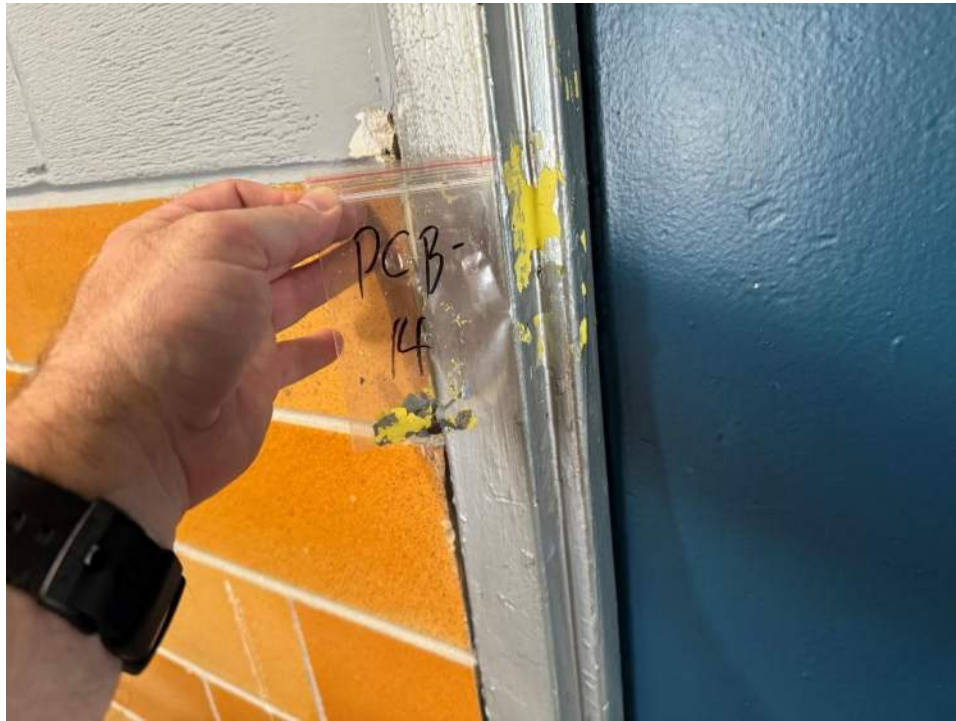
View of the Silver Lead Containing Paint. (PCB-14, 0.026% Pb)
