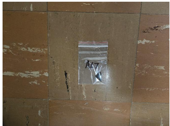
Photo #10 Sample A-67. Employee Home, Asbestos Containing 9" x 9" Floor Tile.
