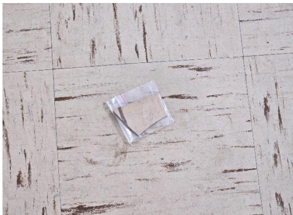
Photo #11 Sample A-68. Employee Home, Asbestos Containing 9" x 9" Floor Tile and Black Mastic.
