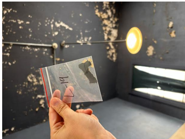
Photo #27 Sample L-19 – Grey Lead-based Paint on Plaster Ceiling in Supply Depot 1 st Floor.
