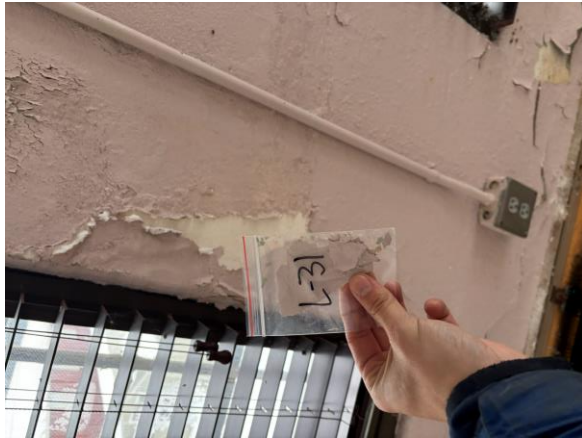
Photo #31 Sample L-31 – Pink Lead-based Paint on Plaster Wall in Larches 2 nd Floor.
