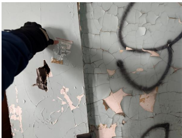
Photo #23 Sample L-6 – Blue Lead-based Paint on Drywall Wall in Oak Hall 2 nd Floor South Connector.
