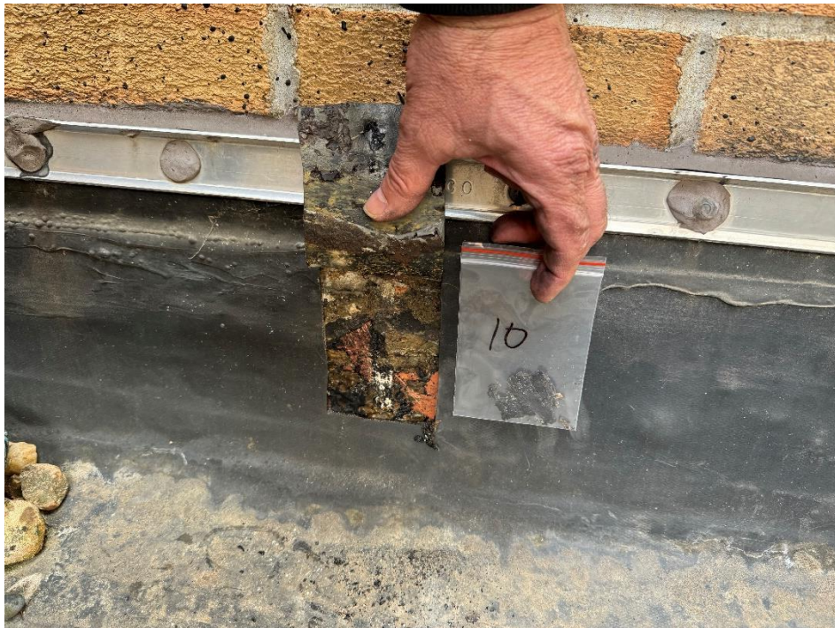
View of the Black Tar and Yellow Mastic on Lower SW Roof section. (NARR-10, 4% Chrysotile in Black Tar, <1% Chrysotile in Yellow Mastic)
