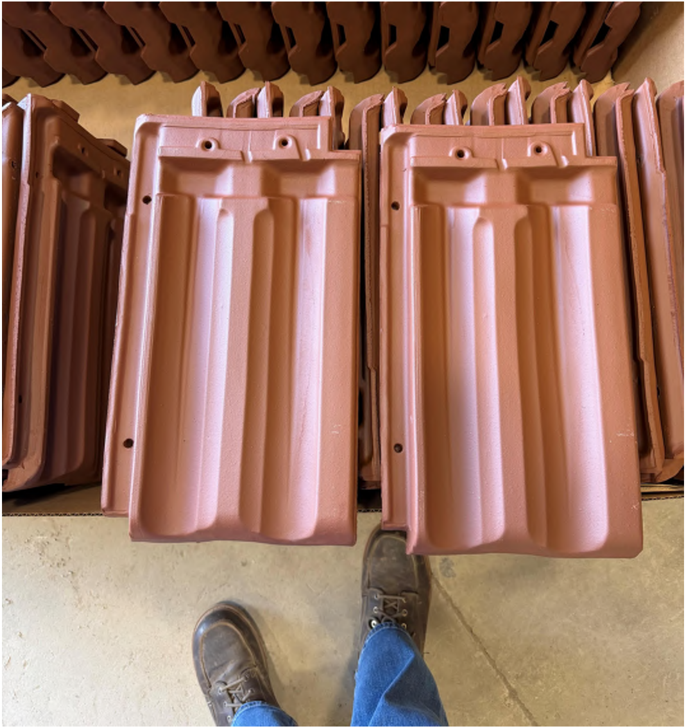
Photograph of the added nail locations in sample test firings
