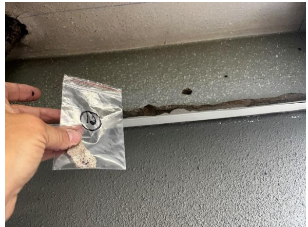
Photo #12 Sample #12 - Old concrete wall layer in Room ED2-16.
