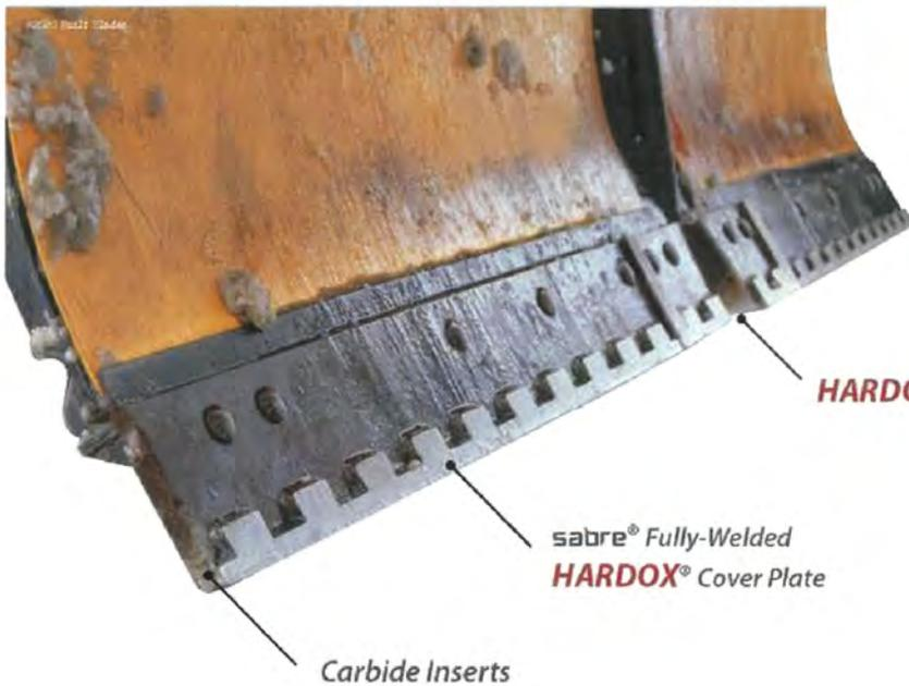
The **sabre® V-BLADE KITS** are designed for simple bolt-on replacement, and built for municipal and heavy-commercial plowing applications. Tungsten-Carbide inserts provide extended wear life up to 10:1 over OEM Steel. Impact-sensitive Carbide Inserts are protected by the **sabre®**'s Light-Weight Fully-Welded **HARDOX®** Cover Plate
