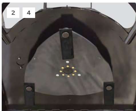
4. ROUNDED FLYWHEEL WITH 3 DOUBLE-SIDED BLADES BOUNCES OFF STUMPS
