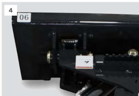
4. FLOATING DESIGN FOR A SMOOTH FINISH & PROVIDES FULL DOWN PRESSURE CAPABILITY
