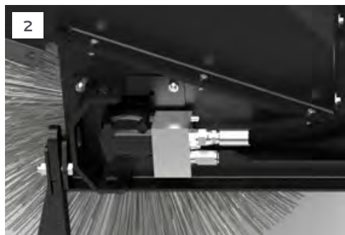
1. SWING LINKAGE SYSTEM SELF-CENTERS BROOM WHEN ANGLED
