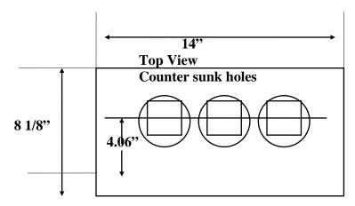
Size; 1" x 14" x 8 1/8" Blade Double Bevel Flat Bolt Size = 3/4" x 2 3/4"
