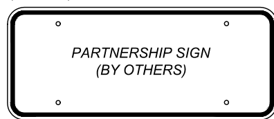
MIDDLE PANEL (1'-8" x 4') 0.080" ALUMINUM SUBSTRATE
