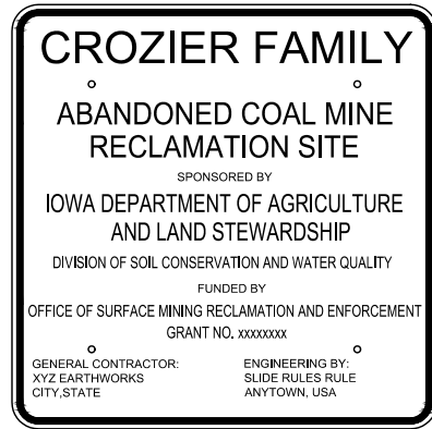
TOP PANEL (4' x 4') 0.080" ALUMINUM SUBSTRATE
