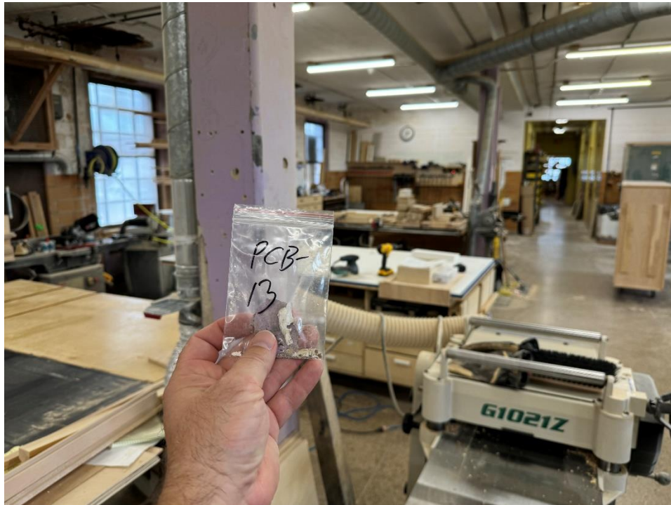
View of the Light Purple Lead Containing Paint. (PCB-13, 0.043% Pb)
