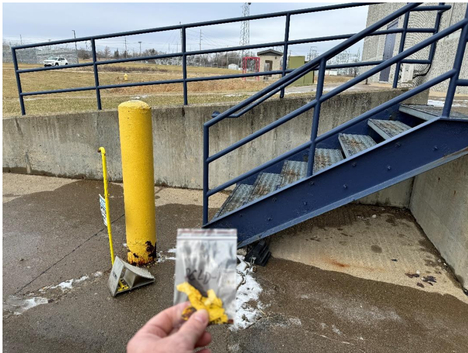
Paint chip sample collected from the NE bollard.
