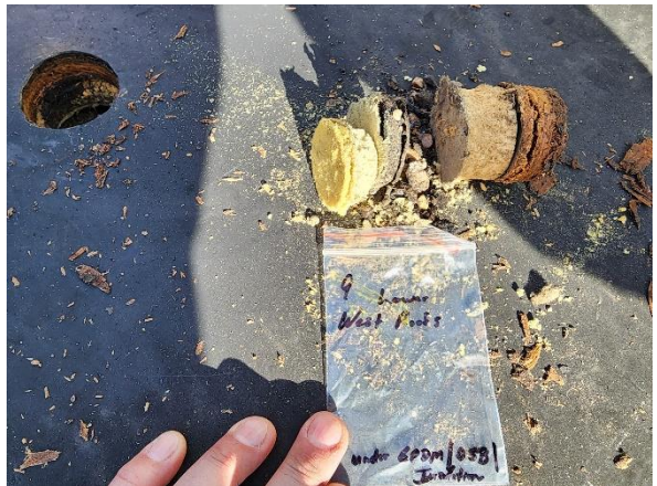
Photo #4 Sample #9. Asbestos containing built-up roofing on lower southwest roof under EPDM/OSB/Insulation.
