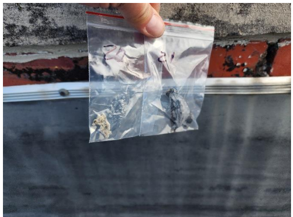
Photo #6 Sample #21. Asbestos containing black-grey roof flashing on parapet walls of upper roof.
