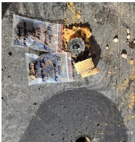
Photo #5 Sample #11. Asbestos containing built-up roofing on lower northwest roof under EPDM/OSB/Insulation.
