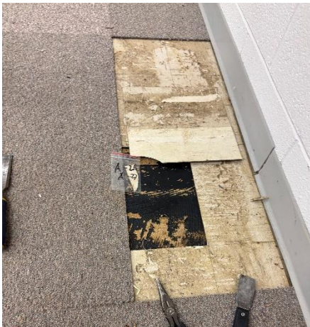
Photo #7 Sample A-26, A-27. Asbestos containing 12" x 12" white floor tile and black mastic.
