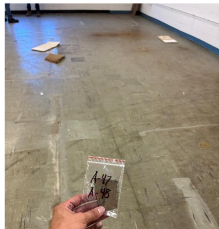
Photo #12 Sample A-47. Asbestos containing 9" x 9" green floor tile and black mastic.
