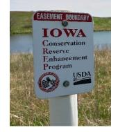
Consultant to provide: T-steel posts, 6-foot tall. PVC sleeve, 4-foot (minimum length) of 2-inch solid PVC pipe. hardware to attach sign.
