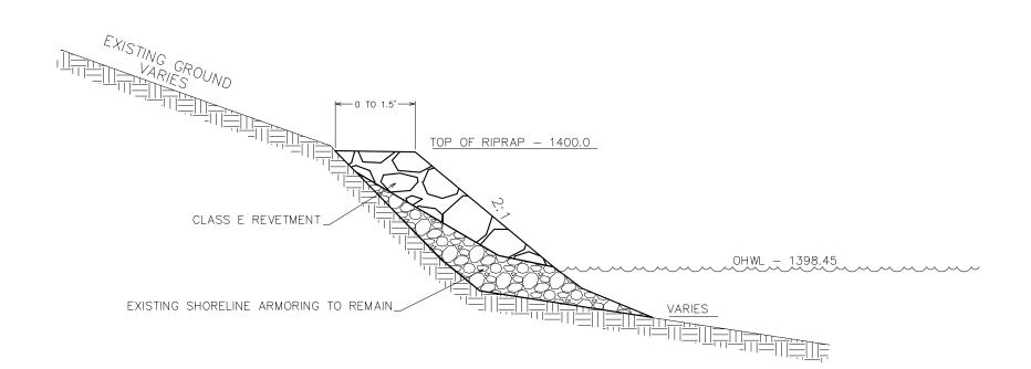
NO EXCAVATION SHAPING OR EARTHFILL WILL BE REQUIRED IN AREAS THAT ARE TO RECEIVE REVETMENT ONLY
