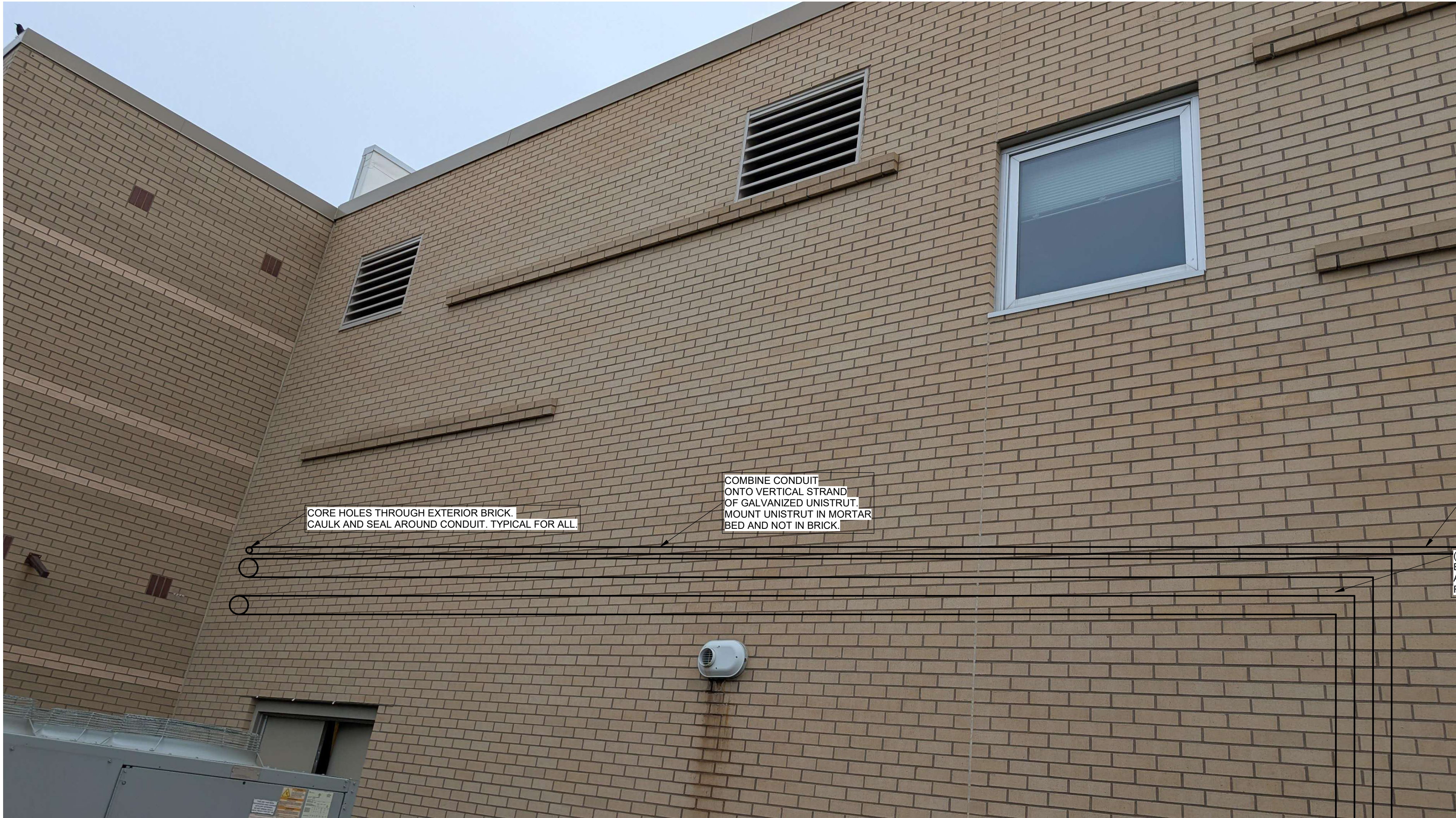
3 CONDUIT ROUTING 1/4" = 1'-0"
