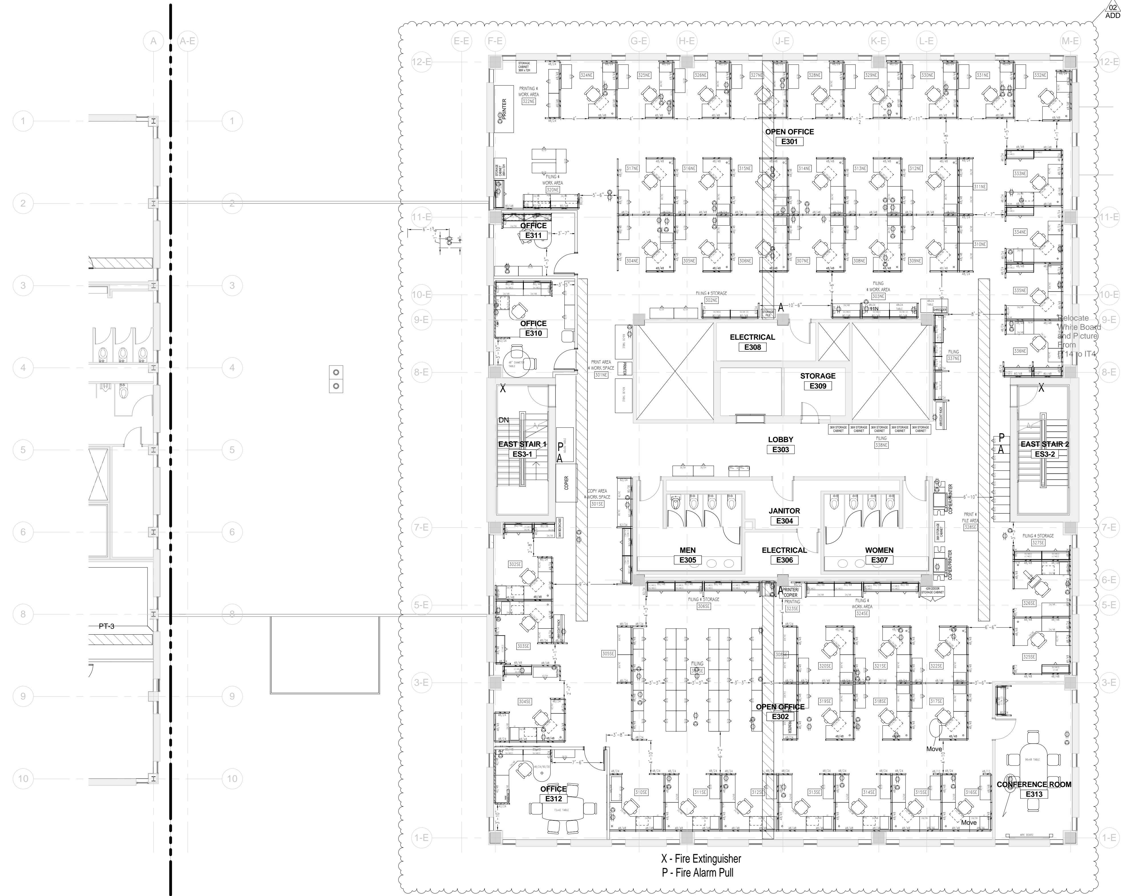
1 LEVEL 3 FURNITURE PLAN - EAST 1/8" = 1'-0" NOTE: FURNITURE PROVIDED AND INSTALLED BY OTHERS - PLANS FOR REFERENCE ONLY. VERIFY ANY FURNITURE COORDINATION ITEMS WITH OWNER.
