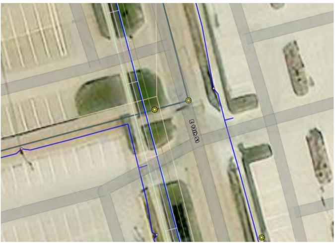
Shows possible communication line running parallel to east side of tunnel, potential waste water on perpendicular to E 13th Street on north side of sidewalk through parking lot island, and possible electrical
