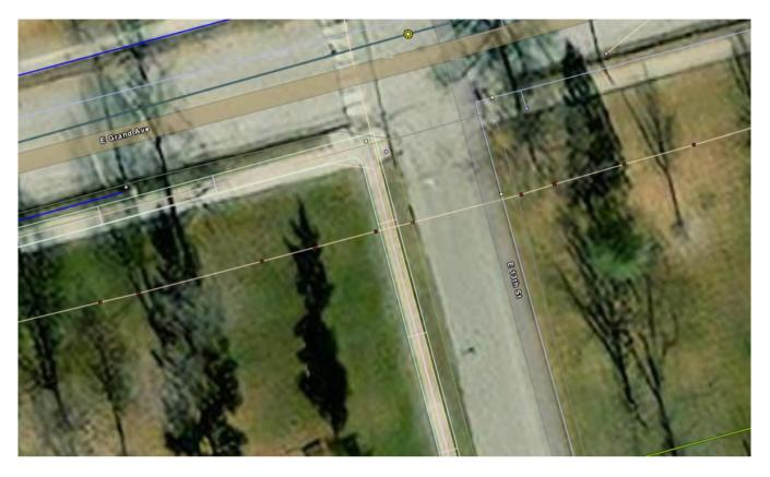
Shows possible natural gas line on south side of Grand Ave and east side of E13th St, possible water line on east side of East 13th St, communications line on west side of E 13th St (to the east of the tunnel), and possible electrical transversing above/below tunnel (main loop?)
