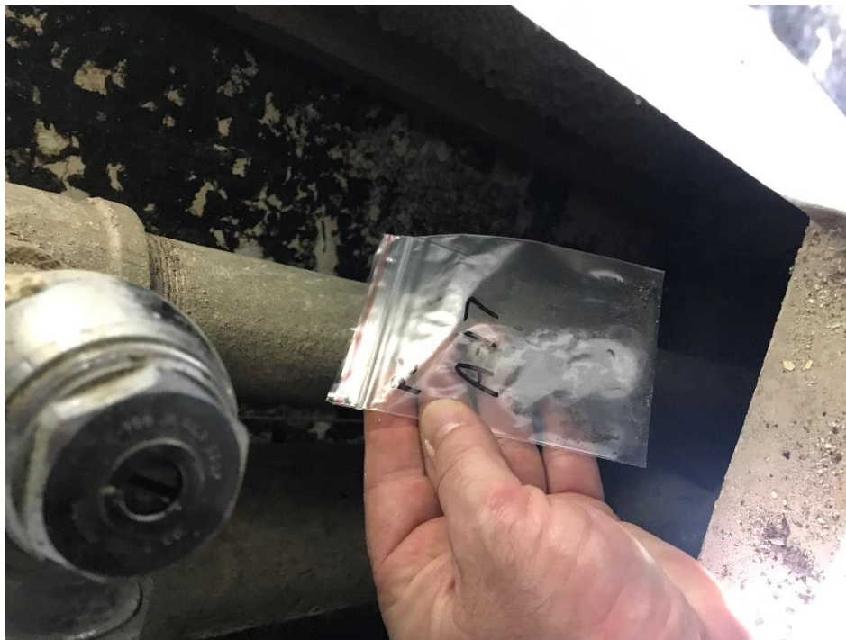
View of the Beige/Gray Lead Containing Paint on Handrails (PC A-16, 0.008% Pb).
