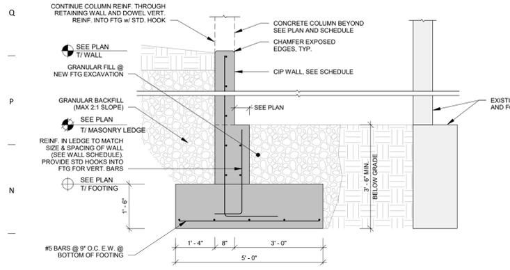
1 RETAINING WALL AND WALL @ EXISTING
