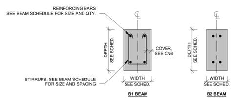
8 CONCRETE BEAM SECTIONS
