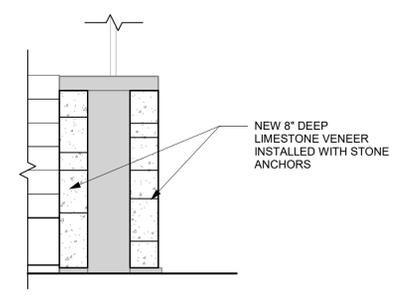
**A12 RETAINING WALL SECTION - NEW WORK**
