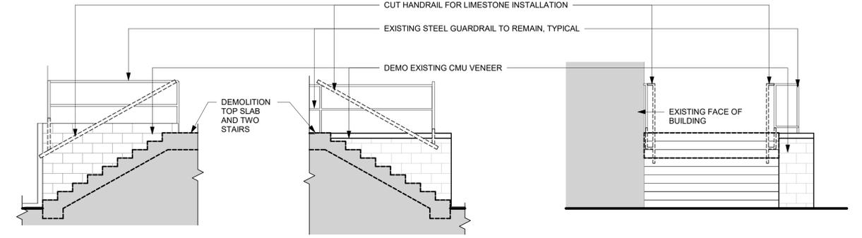
**M12 DEMOLITION STAIR NORTH ELEVATION**
