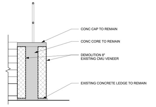
**D12 DEMOLITION RETAINING WALL SECTION**
