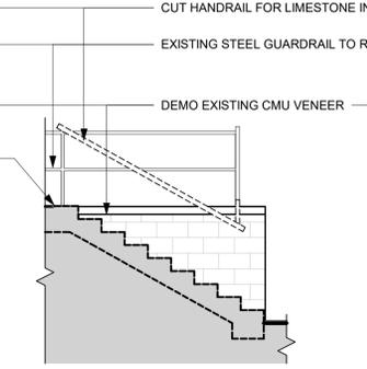
**M15 DEMOLITION STAIR SOUTH ELEVATION**
