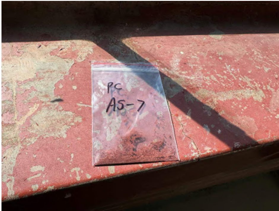
View of the Lead Containing Red Paint. (Appliance Shop Sample: PC AS-7, 0.70% Pb)
