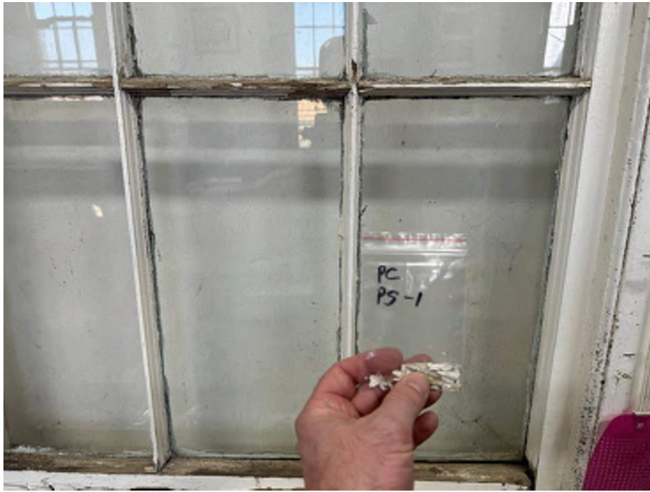
View of the Lead Containing White Paint. (Paint Shop Sample: PC PS-1, 1.3% Pb)
