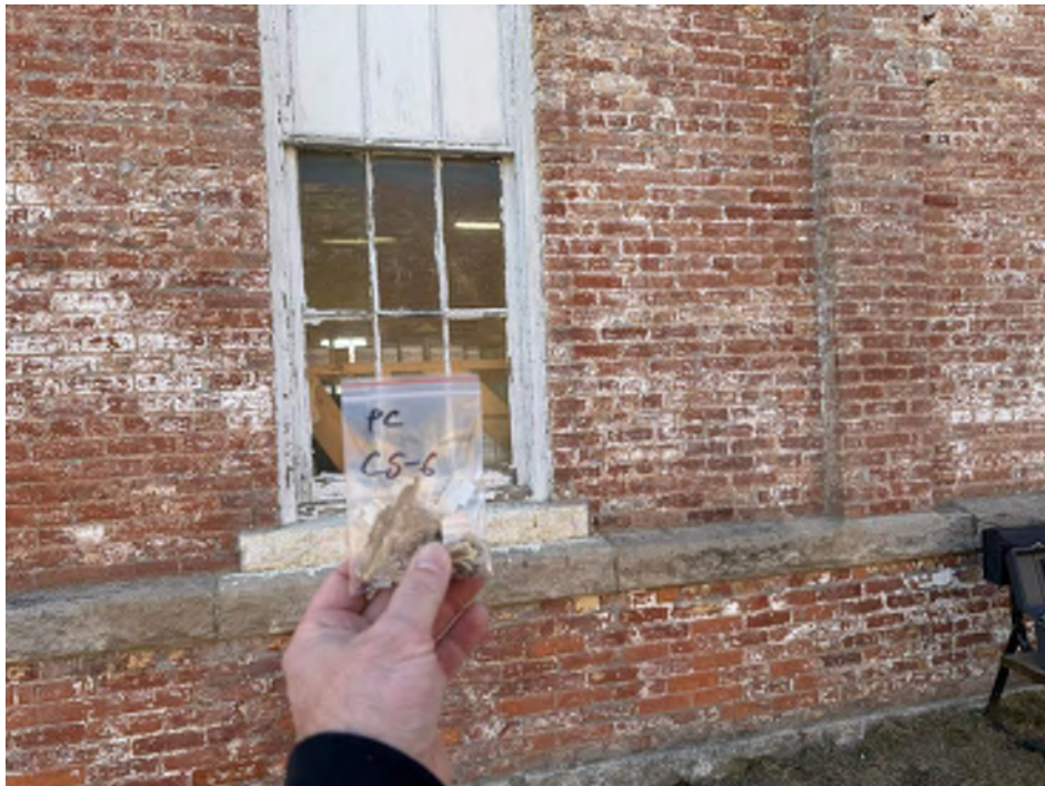
View of the Lead Containing White Paint. (Carpenter Shop Sample: PC CS-6, 12% Pb)
