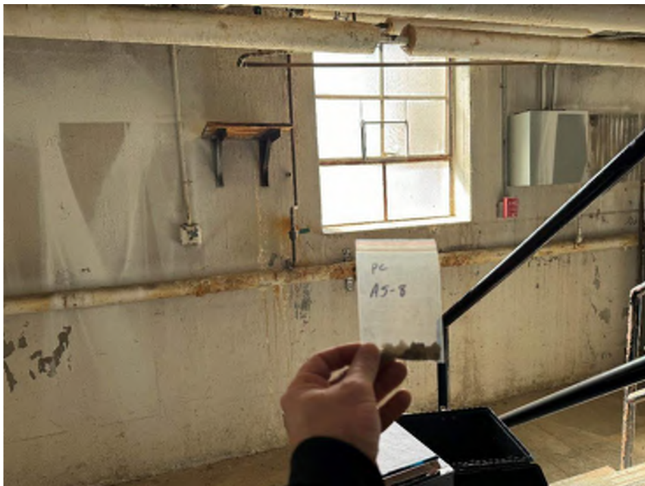
View of the Lead Containing White Paint. (Appliance Shop Sample: PC AS-8, 2.3% Pb)
