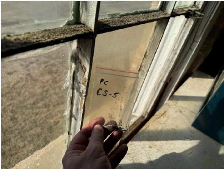
View of the Lead Containing White Paint. (Carpenter Shop Sample: PC CS-5, 10% Pb)
