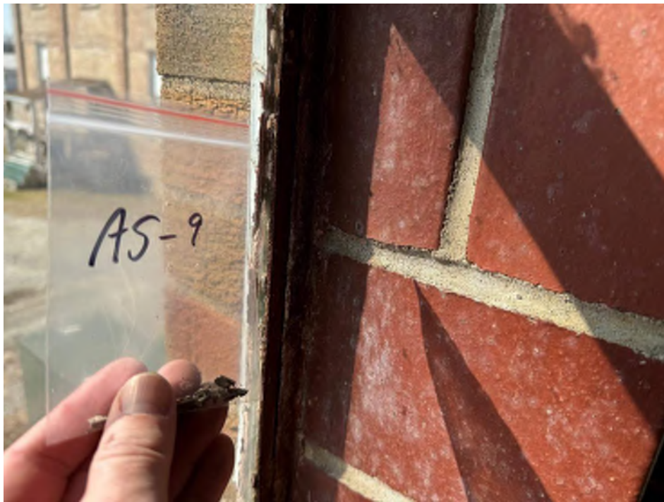
View of the Appliance Shop Window Glazing. (Sample AS-9, 3% Chrysotile)
