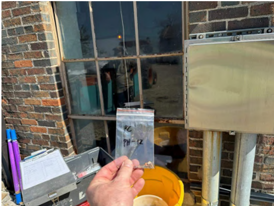
View of the Lead Containing Brown Paint. (Powerhouse Sample: PC PH-12, 9.0% Pb)
