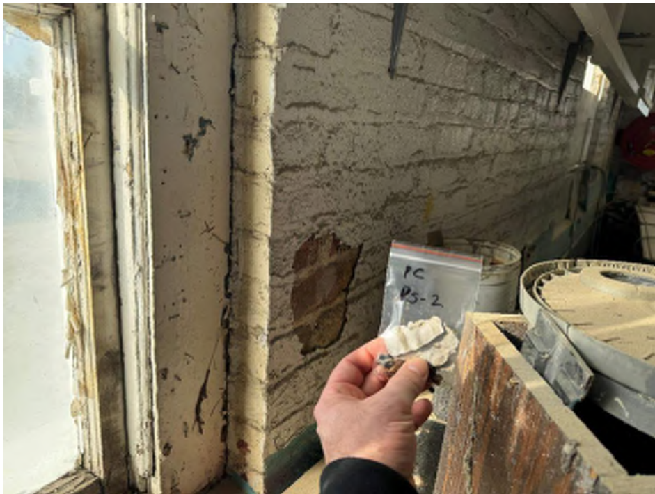
View of the Lead Containing White Paint. (Paint Shop Sample: PC PS-2, 26% Pb)
