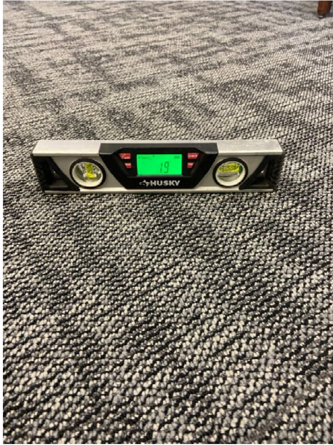
Photo 17: Sloped slab east of room 113
