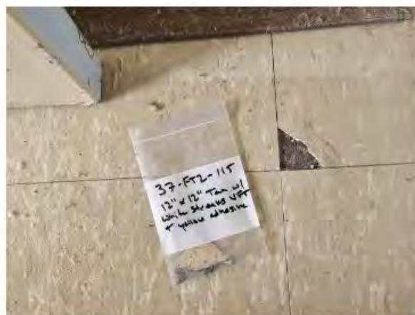
Photo #12 Photo of asbestos containing tan 12-inch by 12-inch VFT with white streaks and non-ACM yellow adhesive HA 37.
