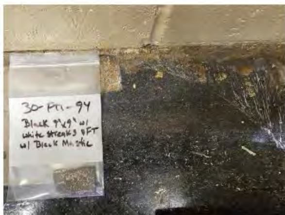
Photo #11 Photo of asbestos containing black 9-inch by 9-inch vinyl floor tile (VFT) with white streaks and associated black mastic HA 30.
