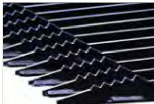
Serrated teeth design allows for better load gripping.
