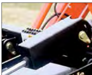
Optional covers protect hydraulic cylinders and fittings.
