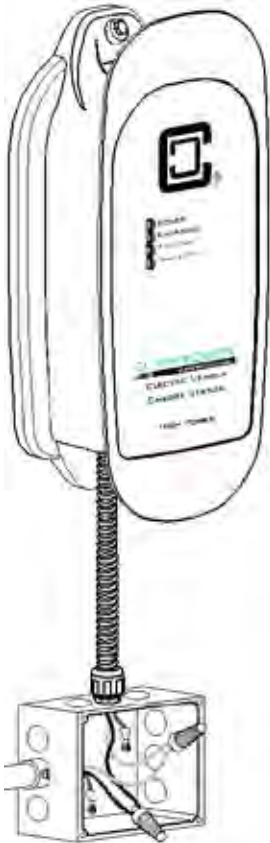
Figure 8. Wiring the HCS in a junction box
