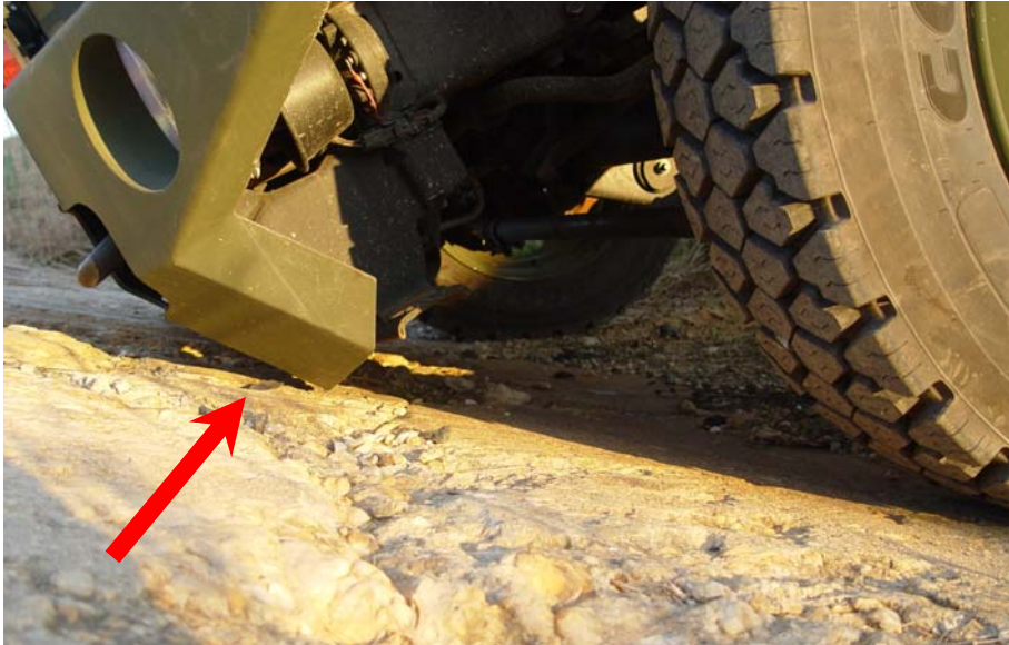
Figure 11. Interference between the front bumper of the BearCat and the wall of the trench crossing obstacle.
