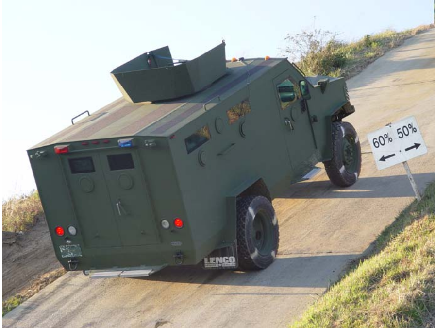
Figure 4. The BearCat ascending the 60-percent longitudinal grade.
