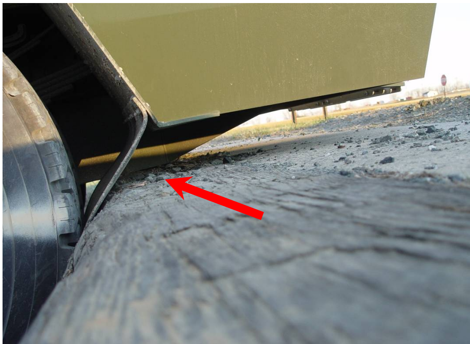
Figure 9. The interference between the fuel tank armor of the BearCat and the top of the 45.7 cm (18 in.) vertical wall.
