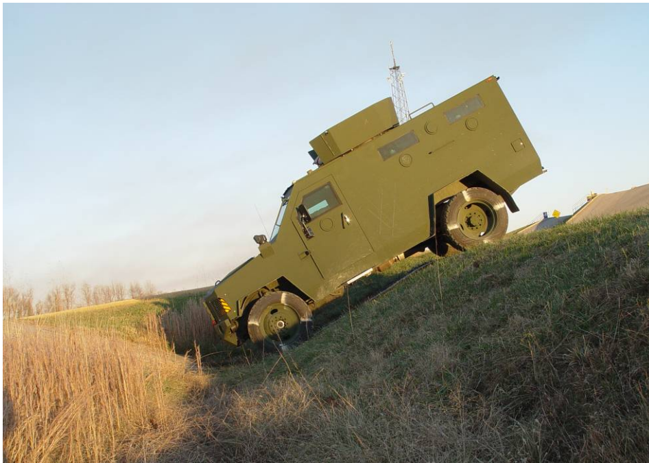
Figure 10. The BearCat negotiating the trench crossing obstacle.
