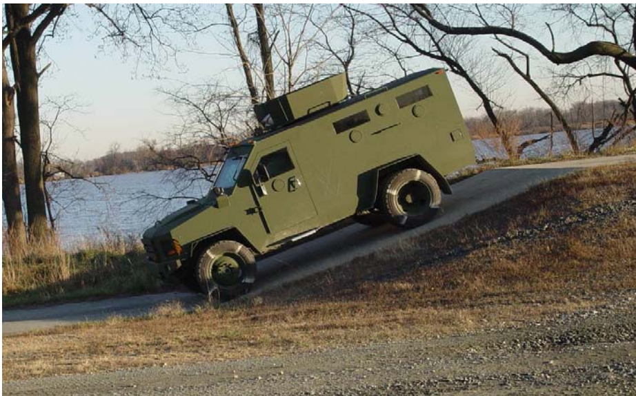
Figure 12. The BearCat negotiating the 15 degree simulated C-130 loading ramp.
