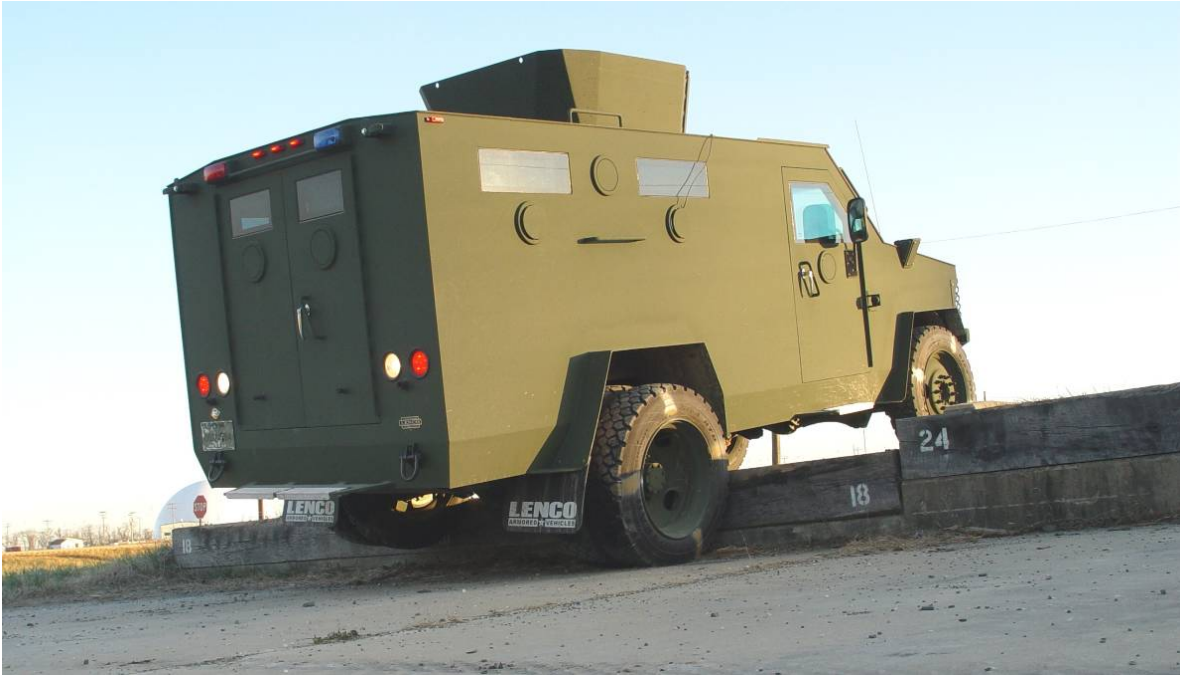
Figure 8. The BearCat negotiating the 45.7 cm (18 in.) vertical wall in the forward direction with the rear axle approaching at an oblique angle.
