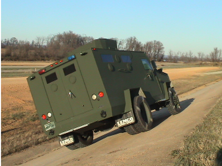
Figure 7. The BearCat negotiating the 40-percent side slope.
