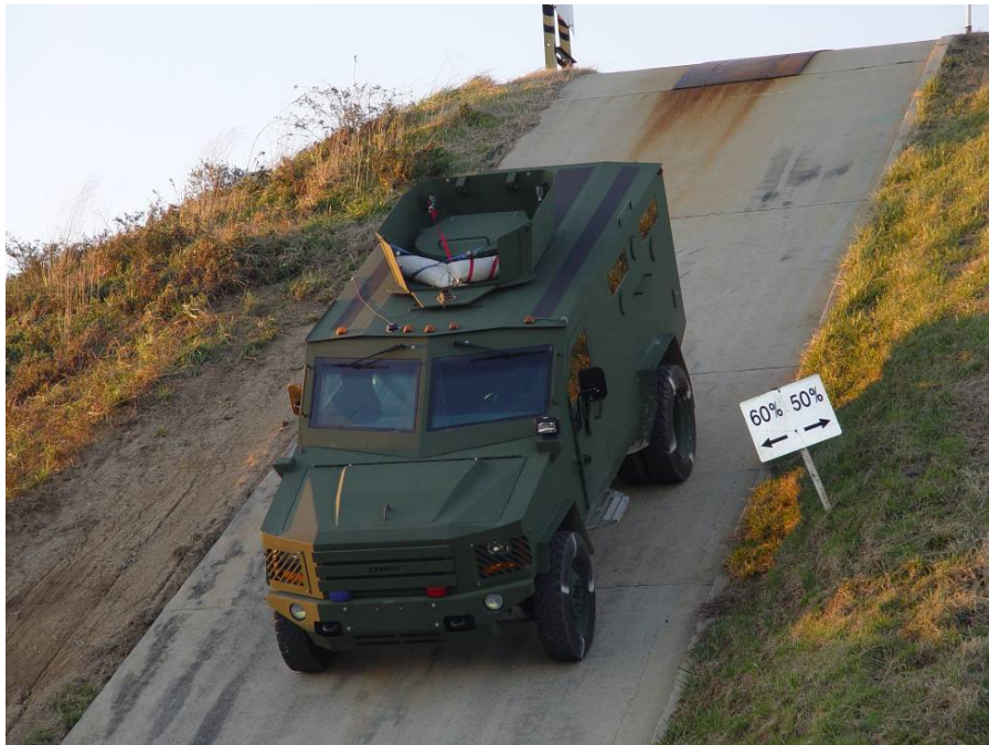
Figure 5. The BearCat descending the 60-percent longitudinal grade.
