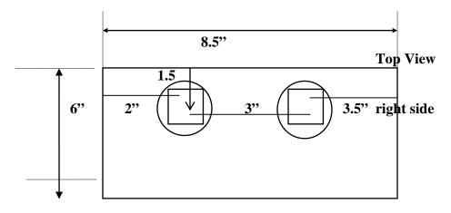
Counter sunk holes Holes are 1 ½" FROM TOP Size; 5/8"x 6" x 8.5" Blade Steel Plate to make curb shoes
